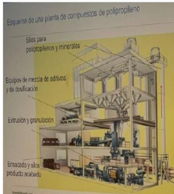
Diagram of a polypropylene compounds plant
